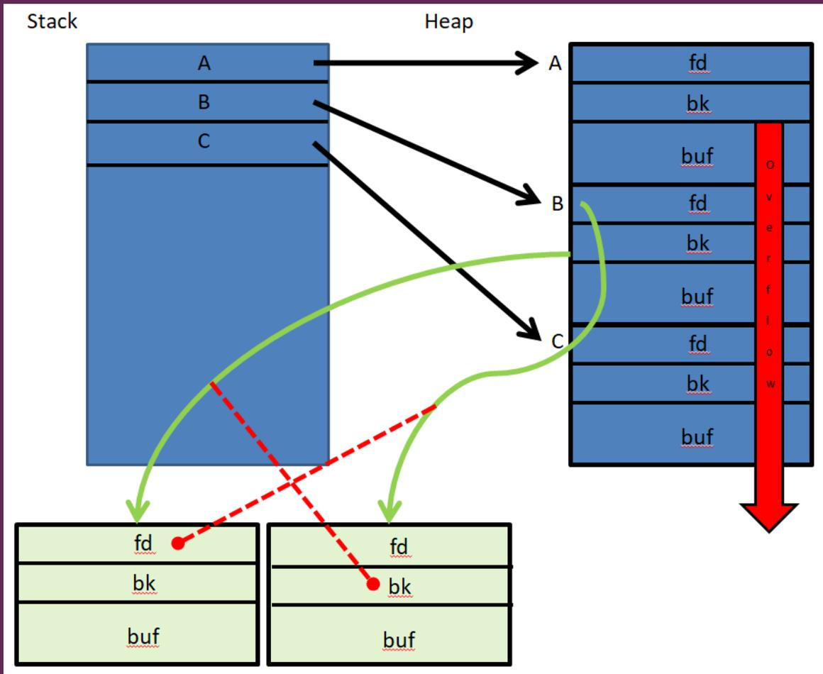
Figure 24: Schema of "unlink" program operation
