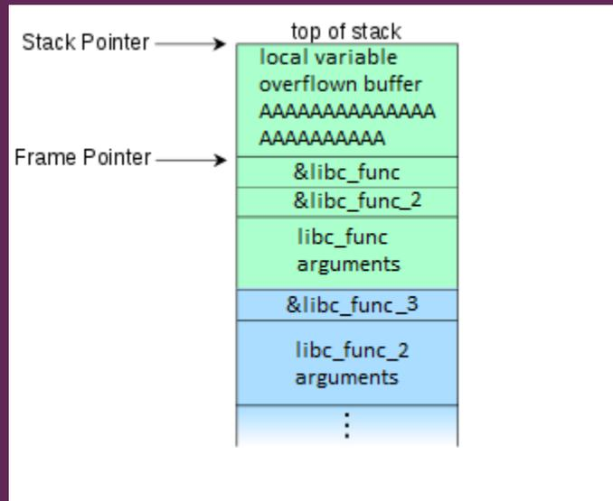
Figure 27: Stack layout after a simple ROP override (i.e. one that doesn't involve repositioning the stack).
