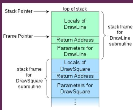
Figure 8: schema of stack frame layout
